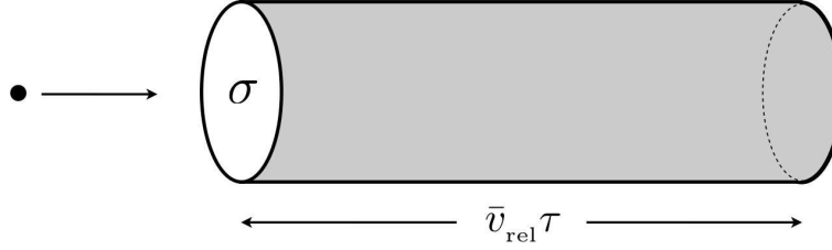
Figure 6.3: Graphic representation of the equation n \sigma \bar{v}_{\text{rel}} \tau = 1 , which yields the scattering time \tau in terms of the number density n , average particle pair relative velocity \bar{v}_{\text{rel}} , and two-particle total scattering cross section \sigma . The equation says that on average there must be one particle within the tube.
